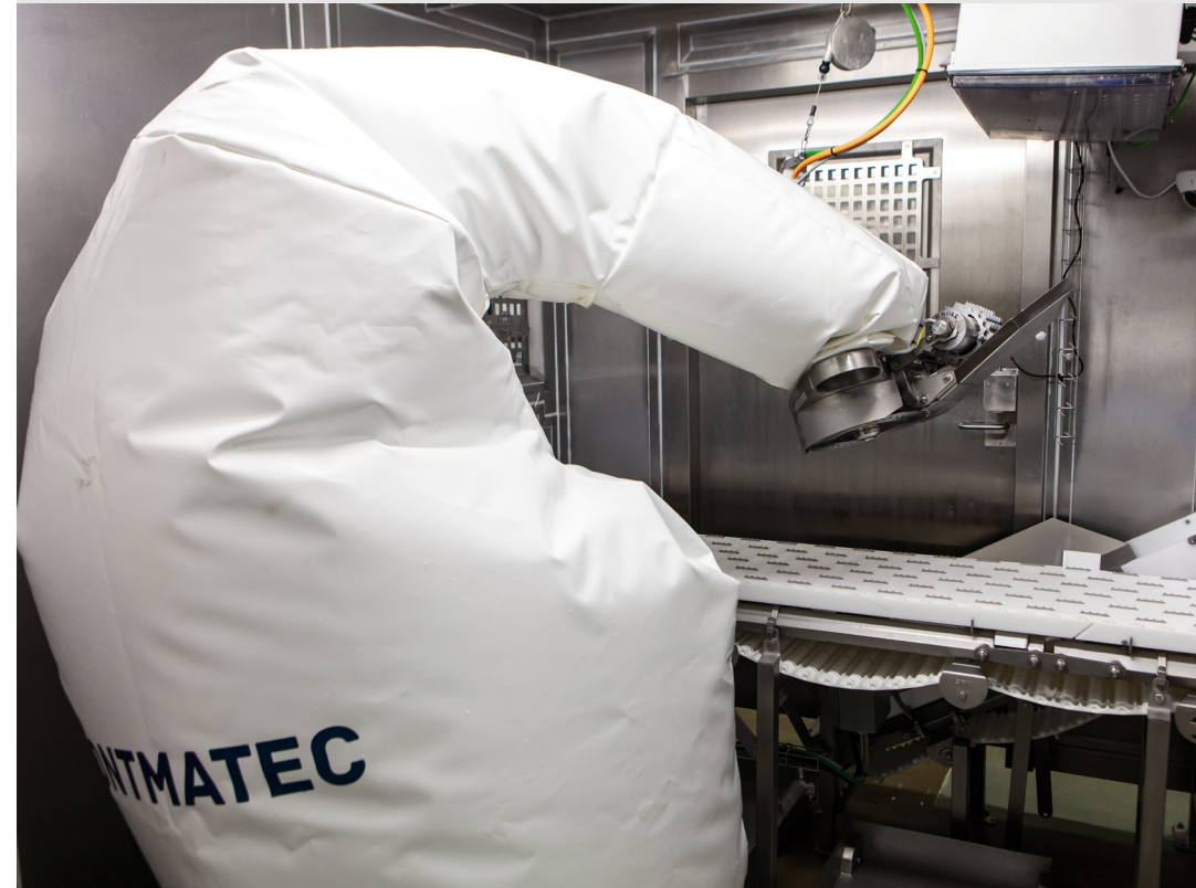
Frontmtec Robotic Chine Bone saw uses a vision system to assess each primal middle for the optimal cut patterns – thus greatly optimizing yield, minimizing waste, and replacing a tedious operation that was traditionally done manually.
