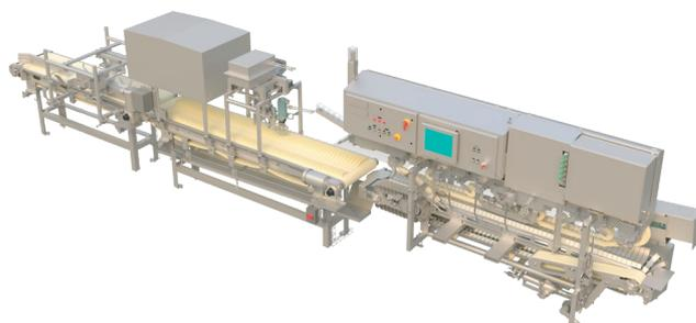
Automatic loin puller, scribe saw and alignment system
