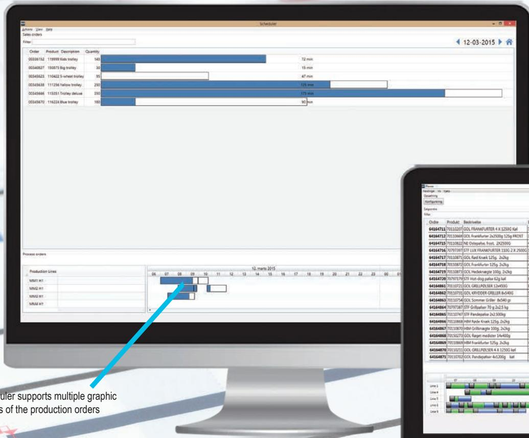
The individual production orders are assigned to the individual production lines and are represented as timelines.
